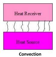
Convective heating relies on the movement of hot fluid or gas, such as air, which acts as a carrier of heat from one body to another. In industry, forced convection is commonly used, that is, the gas or liquid is directed towards the article by a fan or pump. Natural convection occurs because gas or liquid at different temperatures have different densities. An ordinary central heating radiator emits heat mainly through "natural convection".
