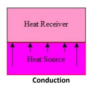
Conductive heating is achieved by placing an article into touch contact with a heat source. The rate of heat transfer is determined by several factors, not just the thermal properties and difference in temperature of the two bodies. The surface conditions over the contact area, the pressure of contact and the nature of any gas, liquid or solid films at the interface all play a part in the conductive process.
