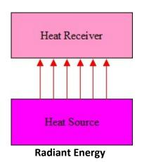
The use of FAR Infrared radiant energy provides certain advantages over conductive and convective heat transfer:
